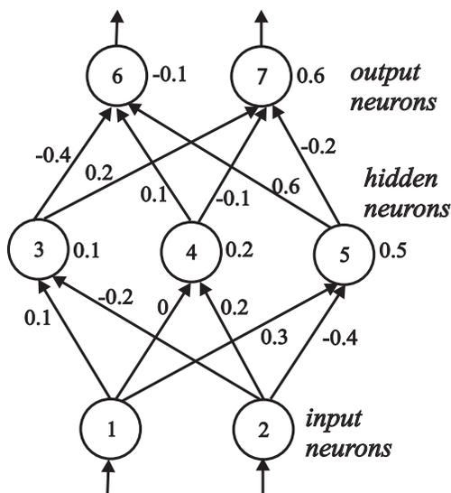
Let the learning rate  $\eta$  be 0.1 and the weights be as indicated in the figure above. Do the forward propagation of the signals in the network using T1 as input, then perform the back propagation of the error. Show the changes of the weights.
