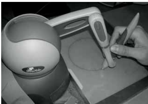
Fig. 1. Experimental Setup showing the Phantom Omni device and a participant drawing a circle.
