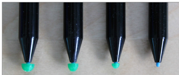
Figure 4. The four nibs used in the Part II of the experiment. From left to right: 5.6 mm, 4.4 mm, 3.5 mm, and 1.6 mm.
