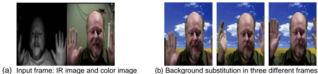
Figure 2: An example of input images and segmentation results of the proposed system: (a) One frame of an automatically synchronized mirrored video pair: IR video and color video, (b) Segmentation results using the proposed algorithm for three different frames.
