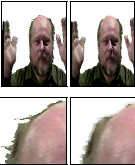
Figure 8: Boundary after segmentation (left), and after border blurring (right).
