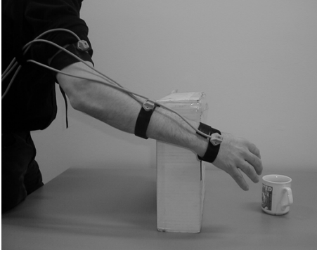
Figure 3. Grasping movement around an obstacle. The movement sensors were placed on the upper arm, the forearm, and the hand.
