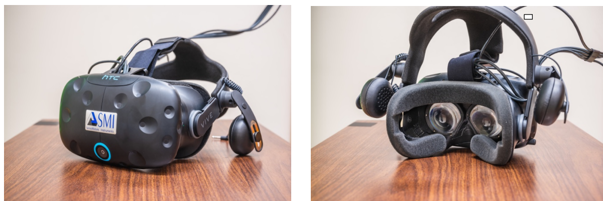
Figure 1: (left) Outside view of HTC Vive HMD. (right) Inside view of HTC Vive HMD with SMI eye tracker. Photos taken by Jacob Gerlofs.
