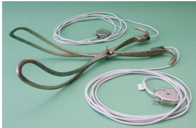
Figure 10: Instrumented forceps with position sensors
