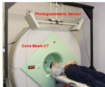
Figure 1: Fusion of CBCT and photogrammetric sensor
