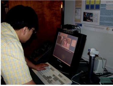
**Figure 5:** Prototype tele-immersive system composed of two synchronized camera, a side-by-side multiplexer, a H323 hardware codex, and an autostereo display from DTI.
