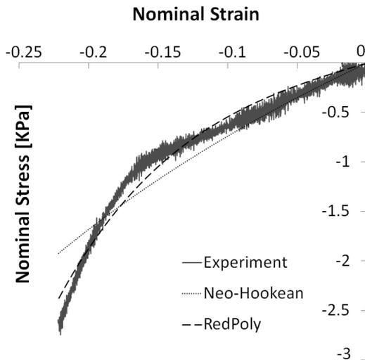
**Figure 4:** Material property estimation using compression test data.
