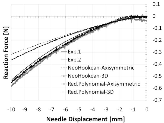
**Figure 5.** Comparison of experimental measurements with FEM simulations for a needle indentation.
