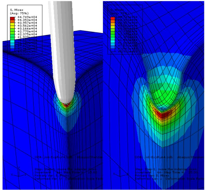
**Figure 7:** Mesh for the axisymmetric (left) and 3D models (right).
