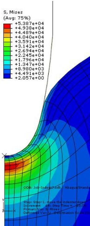
**Figure 6:** Axisymmetrical Indentation in ABAQUS
