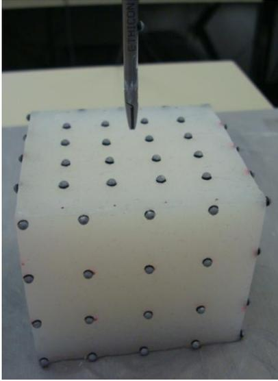
**Figure 2:** Setup for Needle Indentation in a block of 70x80x80 mm. We ensure that velocity was constant and the needle was indented until the strain corresponded to 0.14
