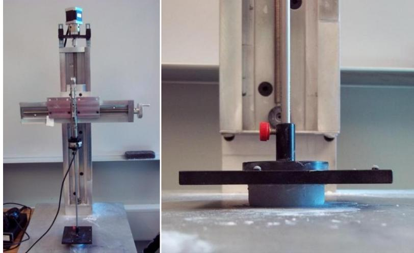
**Figure 1:** Experimental setup for the compression test of a cylindrical shape silicon rubber (Ecoflex -0010). The surfaces were lubricated and the tissue was compressed to a strain of 0.227.
