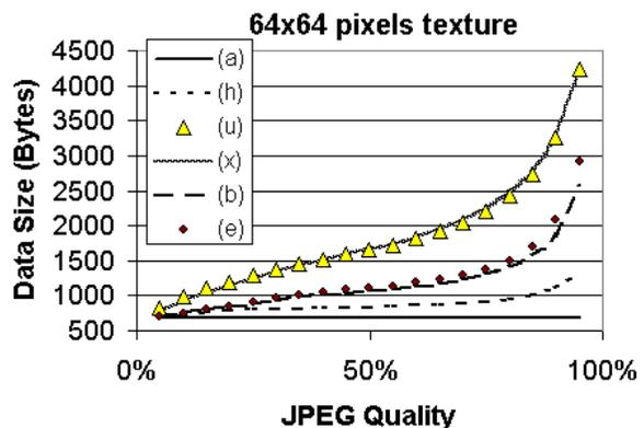
**Fig. 4.1:** JPEG data size relates to quality following an exponential function.
