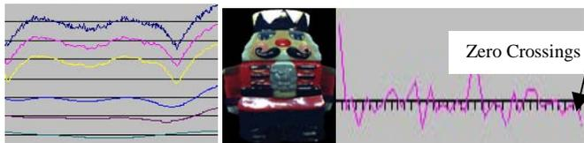
**Fig. 1:** (Left) Starting from the original signal or scale 0, increasing scale  $S_i$  from top to bottom, extracted near the feet of the Nutcracker toy model (middle); and 18 zero-crossings detected using the second derivative of the Gaussian (called Laplacian-of-Gaussian or LoG – Equation 1) for part of the original signal (right).
