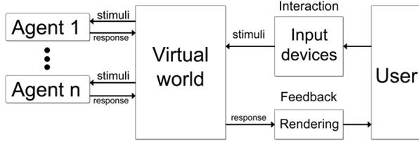
**Figure 2: Layout of the immersive virtual environment**
