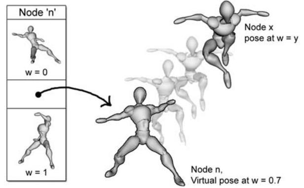
Figure 7: Blended animation from  $Node = x, w = y$  to  $Node = n, w = 0.7$ . As  $n$  only has two poses (at  $w = 0$  and  $w = 1$ ), a virtual pose at  $w = 0.7$  is created
