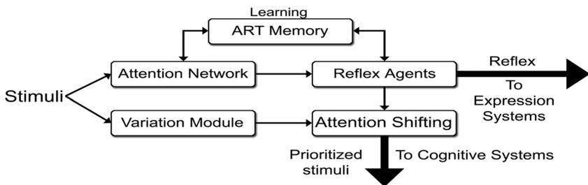
Fig. 2. The architecture of the Perception Layer
