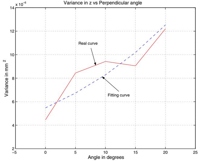
Fig. 6. Variance in  $z$  vs. the incident angle  $\beta$
