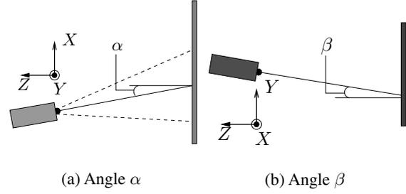
Fig. 2. Definition of the incident angles  $\alpha$  and  $\beta$
