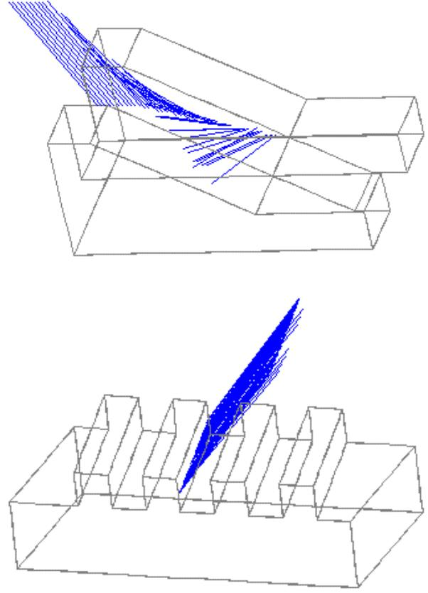
**Fig. 16.** New viewpoints to solve occlusion problems remaining as near as possible to the normal direction
