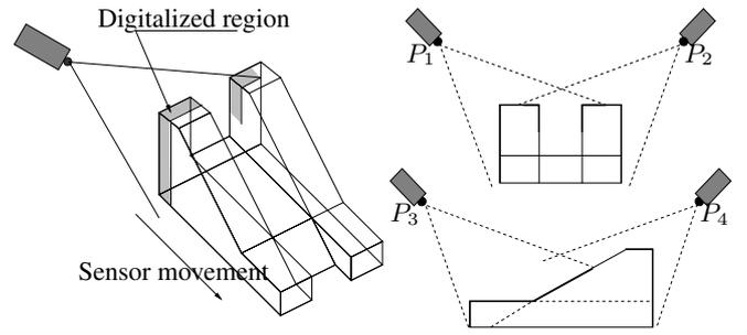
Fig. 19. Standard digitalization process
