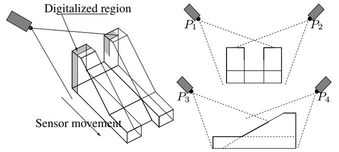
Fig. 19. Standard digitalization process
