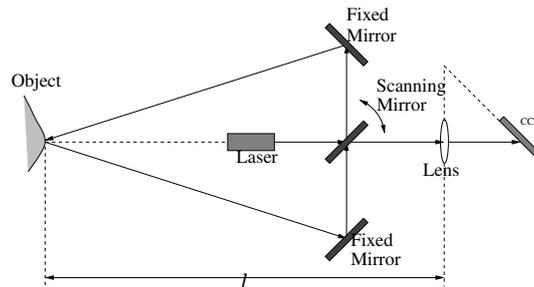
Fig. 1. Optical setup of the NRCC synchronized range sensor
