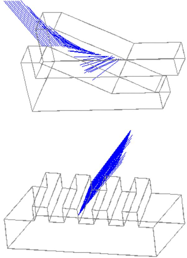
**Fig. 16.** New viewpoints to solve occlusion problems remaining as near as possible to the normal direction
