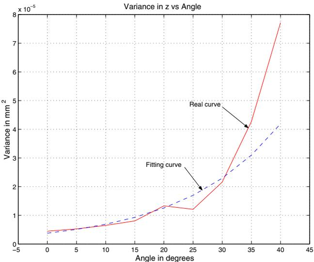
Fig. 5. Variance in  $z$  vs. the incident angle  $\alpha$
