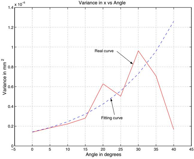
Fig. 3. Variance in  $x$  vs. the incident angle  $\alpha$
