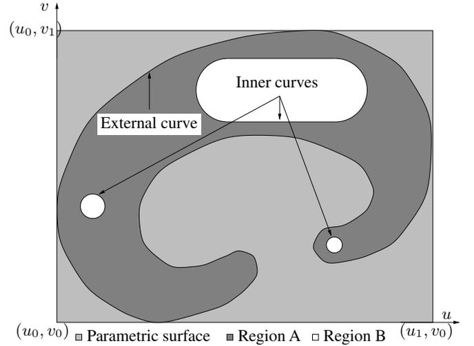
**Fig. 10.** Domain of variation for parameters  $u$  and  $v$
