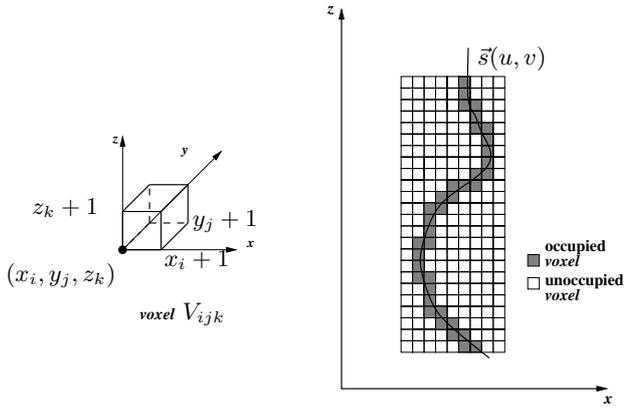
**Fig. 9.** The voxel  $V_{ijk}$  and the voxel representation of the profile of the surface  $\vec{s}(u, v)$
