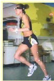
Figure 7: The Vicon motion capture system. Retro-reflective markers are fitted to the subject and tracked as he or she performs the desired movements.
