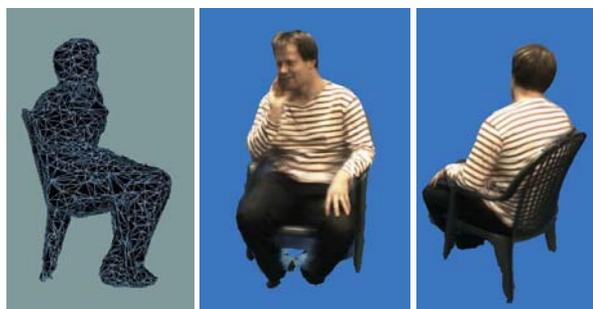
Figure 11: The computed 3D wire-frame model and some textured renderings.
