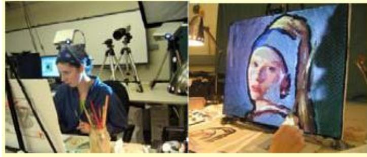
Figure 6: A projector based system for training novice painters. Left: the setup with two projectors and a video camera. Right: a projector-based augmentation showing paint layering.
