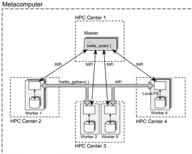
**Figure 1. Programming System Execution Environment**
