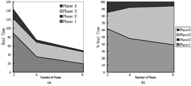
**Figure 10. Breakdown execution time of PSRS application with default `ssh`. (a) phase-by-phase with real time. (b) phase-by-phase with percentage of real time.**
