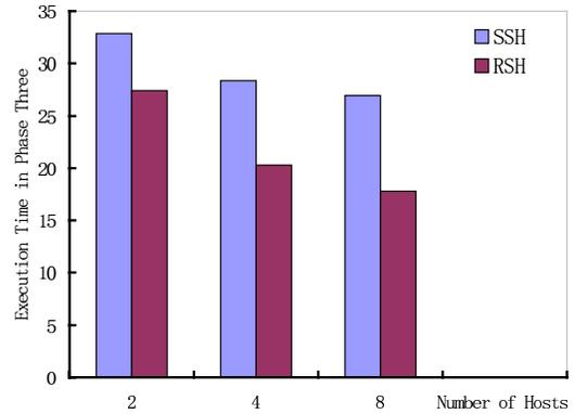
**Figure 12. Overheads of the programming system in PSRS with different underlying communication mechanism**
