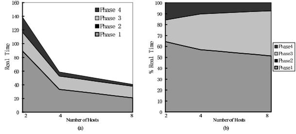
**Figure 11. Breakdown execution time of PSRS application with `rsh` enabled in phase three. (a) phase-by-phase with real time. (b) phase-by-phase with percentage of real time.**
