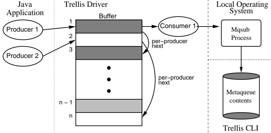
**Figure 2. Bounded Buffer with Per-Producer Links**
