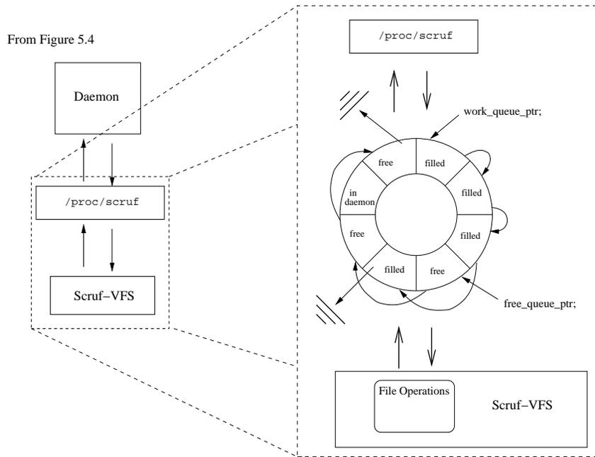
Figure 5.5: The Bounded Buffer used in Scruf-VFS
