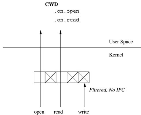
Figure 5.25: An Example of Scruf's Filtering Mechanism
