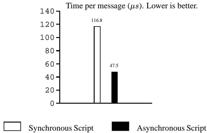
Figure 6.2: Synchronous v. Asynchronous Scripts: Sending 100,000 Messages
