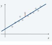
$$-L: y=ax+b \quad \text{Error}(L,p)=\sum_{i=1}^{n}(y_i-ax_i-b)^{n}$$
