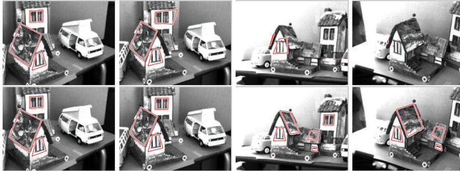
**Fig. 2. Top** Tracking individual patches using a homography. Not all regions can be tracked though the whole sequence and occlusion is not handled. **Bottom** Through the 3D model each region motion is rigidly related to the model, and tracking succeeds through the whole sequence. The model also allows detection and removal of occluded regions and introduction of new regions. See supplied `video1`
