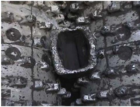
Fig. 6. Close-up of a shoveler's missing tooth stuck in the oilsand crusher. Image from Syncrude Inc.
