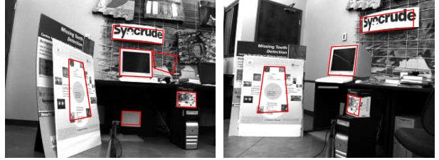
Fig. 3. Tracking planar patches. The model also allows detection and removal of occluded regions.
