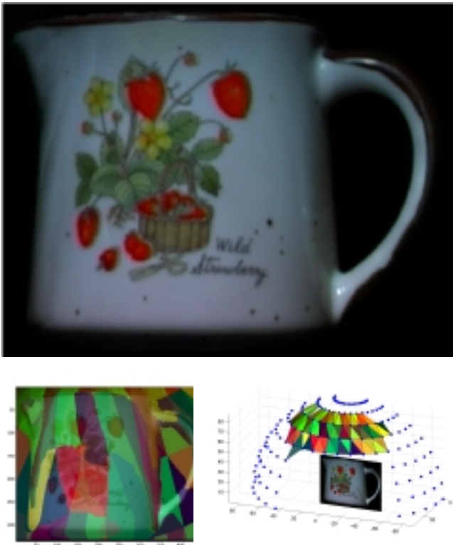
Figure 5: To render the image of the cup, top, from a point light source located 23 cm away, intensities from a number of images in the object's dataset were interpolated. The lower left image color codes each pixel in the rendered image with the triplet of light sources whose corresponding images were used to render that pixel. On the bottom right, the corresponding triplets of light source positions are shown. The dots on the sphere denote the light source positions. The color triangles denote triplets of light source positions. The three images acquired by the three light source positions in the triplet are used to render the intensities of the like-colored regions in the synthetic image, bottom left and top.
