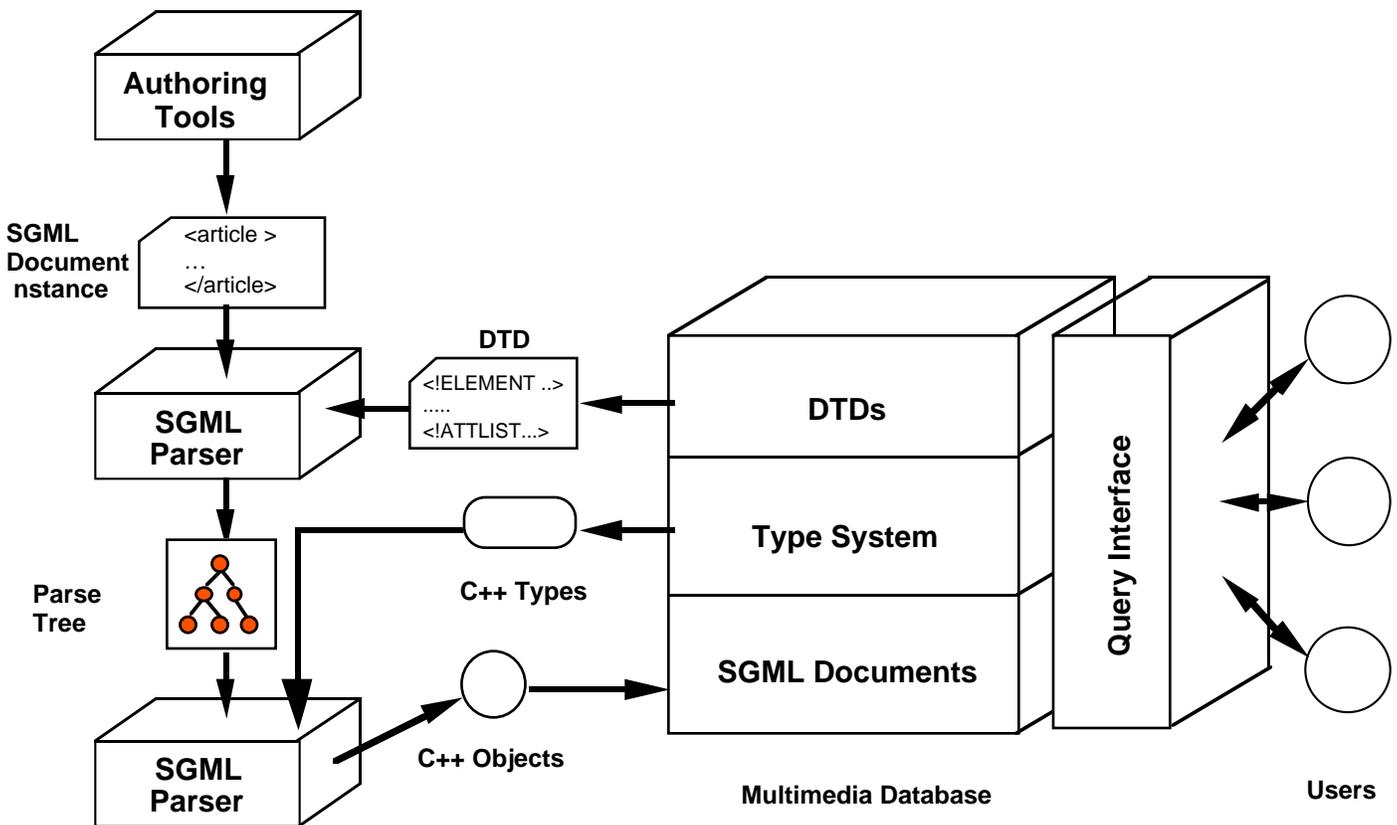
Figure 6. Architecture for automatic document entry
