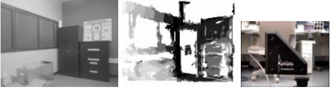
Figure 4.7: Example of a disparity map computed using the Triclops vision system. (a) left intensity image (b) disparity map (c) Triclops device
