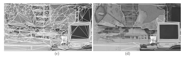
Figure 4: Planar region segmentation: (a) Original image; (b) Edge detection and linking; (c) Constraint Delaunay triangulation; (d) Merged planar regions
