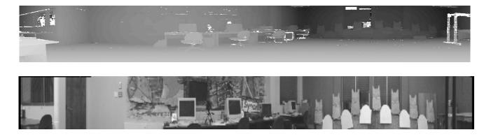
Figure 3: Spherical representation of the range data from an  $180^{\circ}$  scan after filtering (top). Corresponding  $180^{\circ}$  panoramic image mosaic (bottom).
