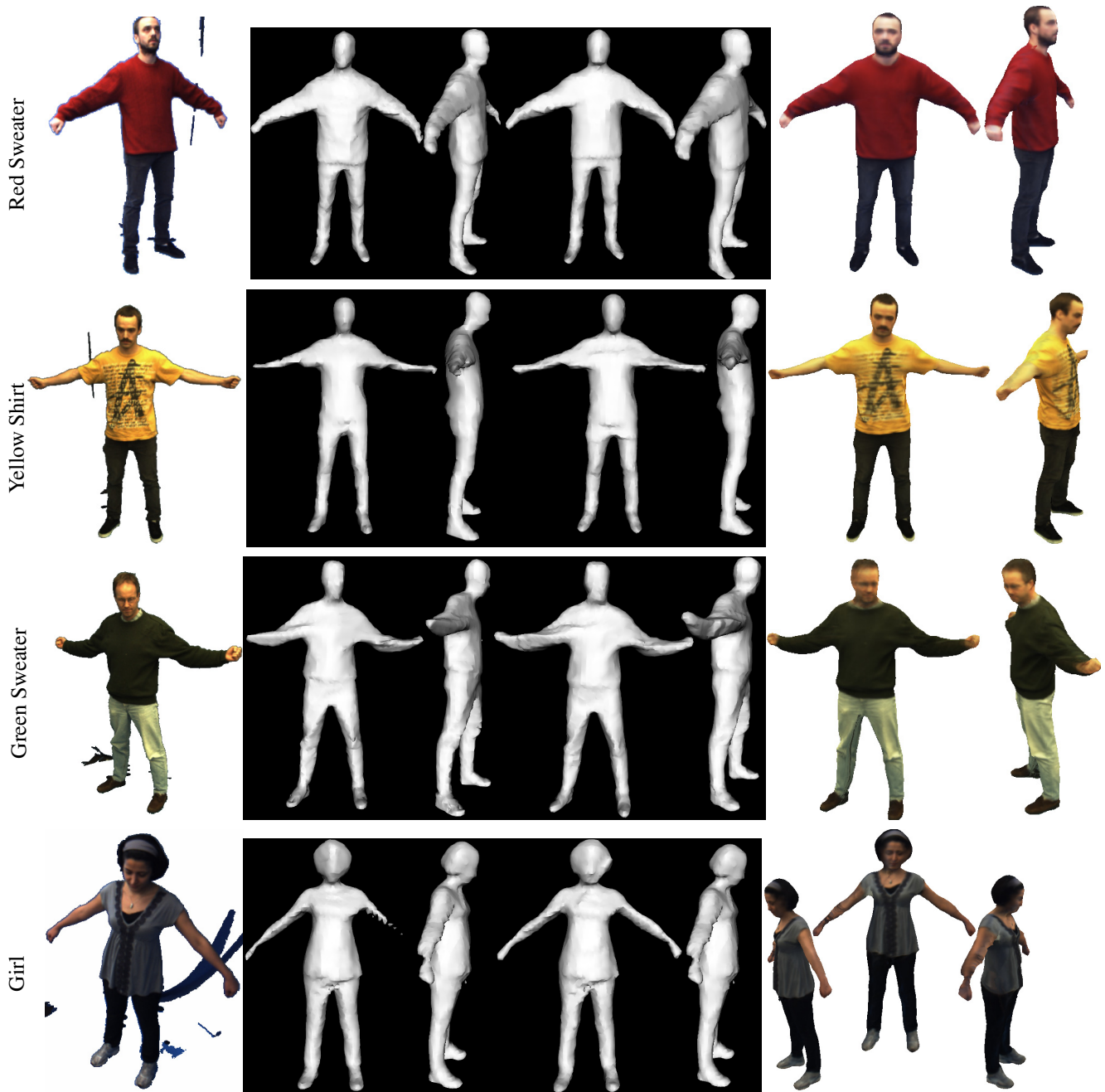
Figure 9. Sample input image, reconstruction without motion compensation (e.g., SFS), the refined model, and a textured model (single average texture).
