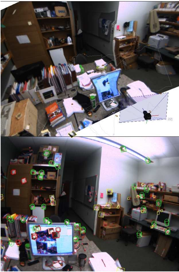
Figure 1. User interface. On top: 3D reconstruction with current camera estimate, trajectory and indication of saved frames. Bottom: live video with tracking markup.
