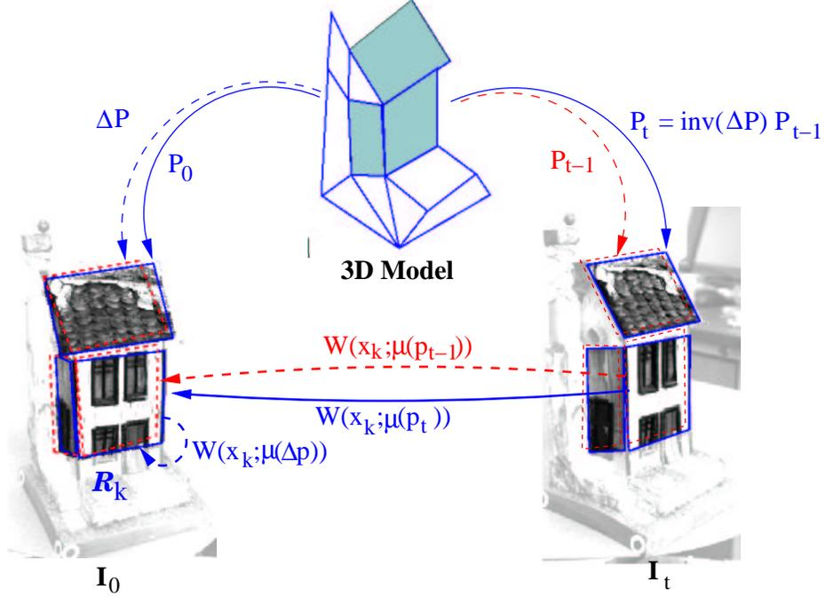
**Fig. 1.** Overview of the 2D-3D tracking system. In standard SSD tracking 2D surface patches are related through a warp  $W$  between frames. In our system a 3D model is estimated (from video alone), and a global 3D pose change  $\Delta P$  is computed, and used to enforce a consistent update of all the surface warps.
