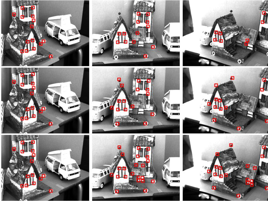
**Fig. 3.** **Top** Translation tracking of individual regions [8, 9]. Though the video sequence many patches are lost. **Middle** A projective 3D model is used to relate the regions, and provide more stable tracking through the whole sequence. **Bottom** An Euclidean model relates the region, and also allow the introduction of new regions. *video2* [1]
