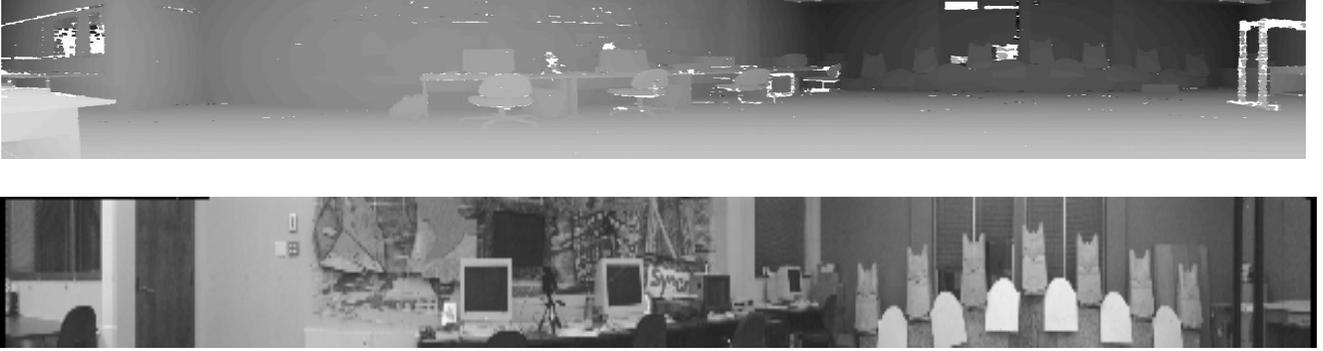
Fig. 2. (top) Spherical representation of the range data from an 180° scan after filtering (bottom) Corresponding 180° panoramic mosaic.
