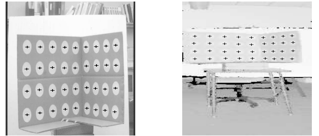
Figure 5: Image of the calibration pattern and the corresponding laser amplitude image. The extracted feature points are marked with '+'
