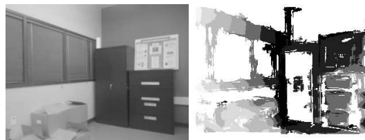
Figure 1: Intensity and disparity image provided by Triclops. In the disparity image: white - no disparity value; dark - far objects; light - close objects
