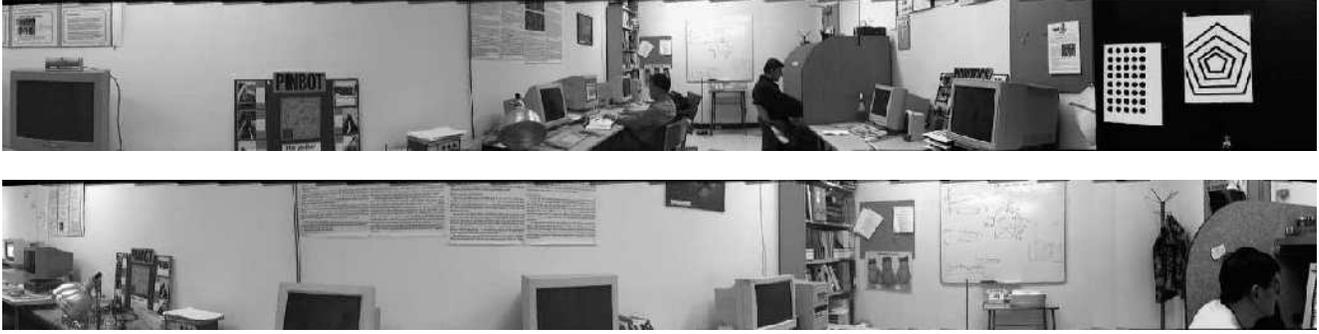
**Figure 5.** Two cylindrical panoramic images (each formed using 25 planar images sampling 180 degrees)
