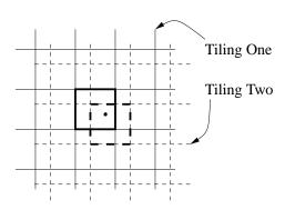
Figure 6.2: An example of tile coding a two dimensional space with two overlapping tilings.
