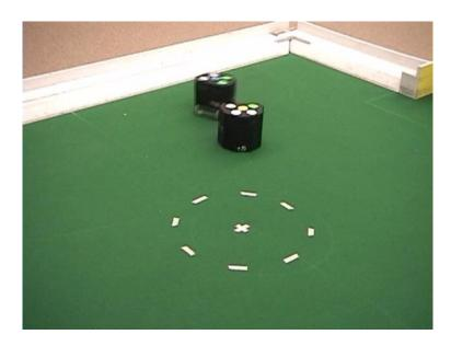
Figure 6.1: Keepout: an adversarial robot task. The top robot is trying to get inside the circle while the bottom robot is trying to stop it.
