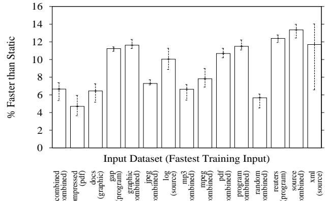
**Figure 9. Static vs. FDO Inlining performance: `bzip2` on Itanium**
