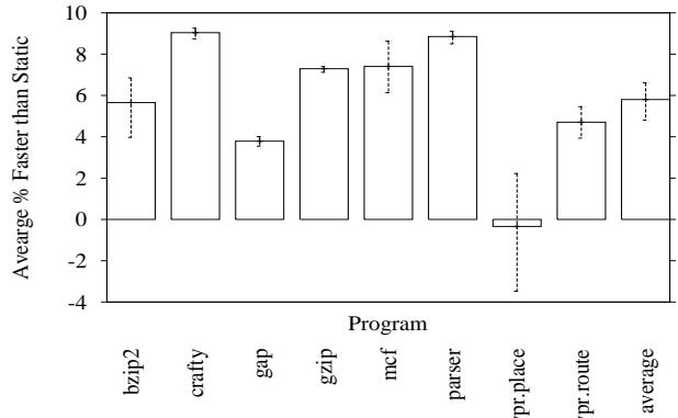
**Figure 7. Average FDO inlining performance on Itanium**
