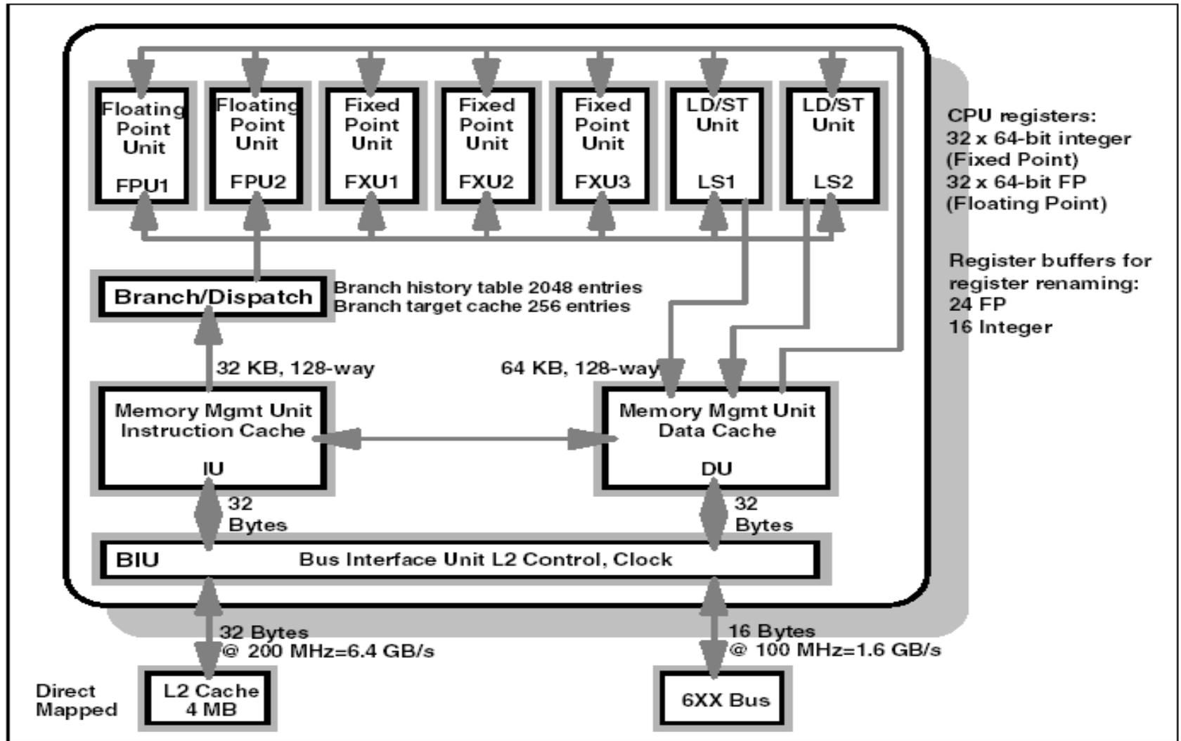
Figure 3. Model 170 - POWER3-II 400 MHz Block Diagram
