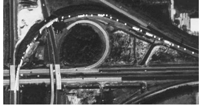
Fig. 12. Example of low efficient road tracking caused by complex road condition. The road tracking starts from the lower left corner of the image. White line segments are the human input, and white dots are the tracking result. Due to the complexity of the road, intensive human input is required.
