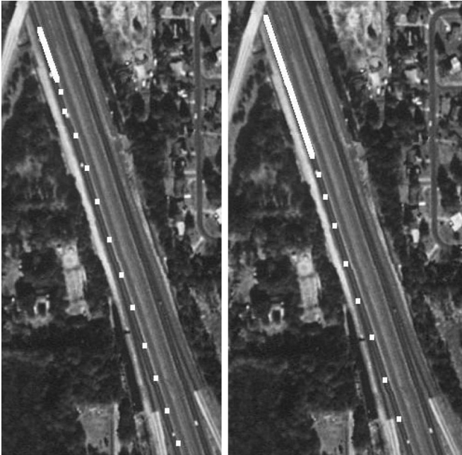
Fig. 11. Example of accurate and inaccurate tracking on the same road. White line segments are the inputs from two users, and white dots are the detected road axis points. In the left image, the input is not at the center of the road. It generates a biased road profile predictor, which in turn makes inaccurate road tracking that is deviated from the true road centerline. The right image shows an accurate road tracking initialized by an accurate human input.
