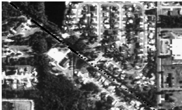
Fig. 11. Road tracking from upper left to lower right. Black dots are the detected road axis points, blackline segment shows the location of human input. This is an extreme case when trees occlude the road. Intensive human inputs are required.
