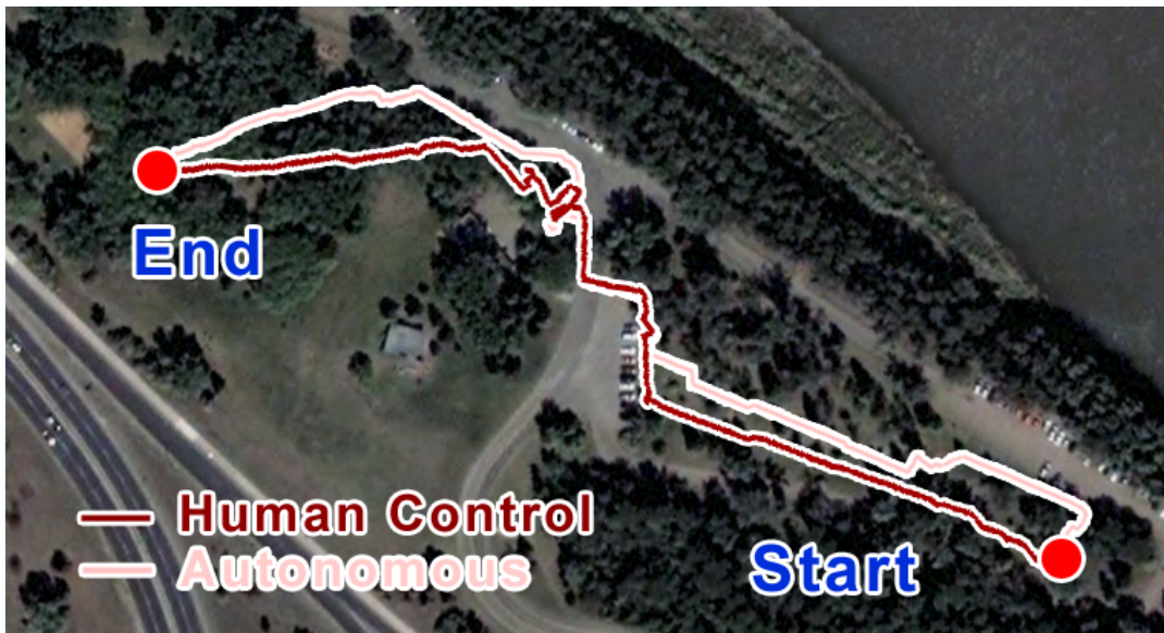
Figure 5: Comparison of two paths in the park test site. The dark path was followed by a human expert teleoperating the robot. The lighter path was followed by the robot under autonomous control. Map image courtesy of Google Maps™.
