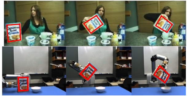
Fig. 1. Sequence showing both the robot and human user performing identical tasks of pouring cereal in a bowl under normal light settings. The red rectangle shows the tracking result on the sequence using ESM [12]
