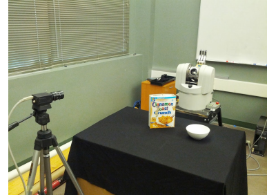
Fig. 2. Set up for recording videos under normal light using a WAM arm and a Barret hand.
