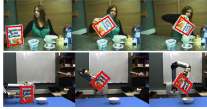
Figure 1: Sequence showing both the robot and human user performing identical tasks of pouring cereal in a bowl under normal light settings. The red rectangle shows the tracking result on the sequence using ESM [11]
