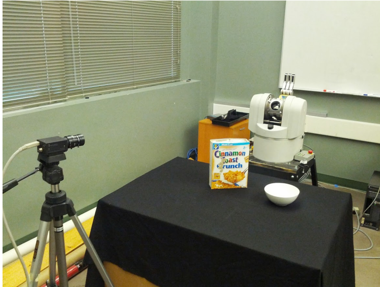
Figure 2: Set up for recording videos under normal light using a WAM arm and a Barret hand.
