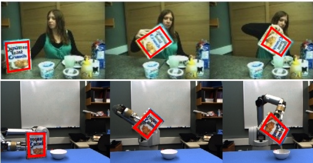
Figure 2.5: Sequence showing both the robot and human user performing identical tasks of pouring cereal in a bowl under normal light settings. The red rectangle shows the tracking result on the sequence using ESM [9]
