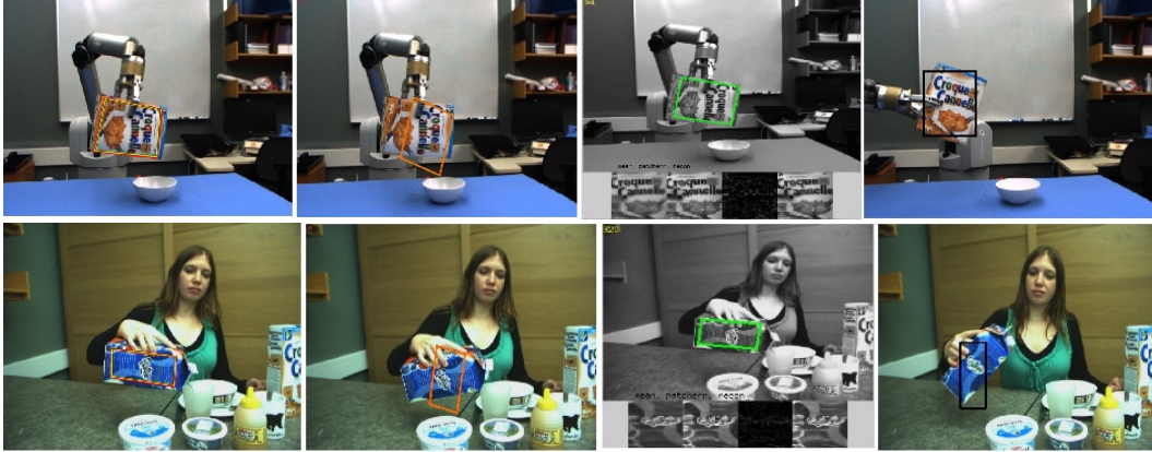
Figure 5.1: L1-APG (orange) [56] and TLD (black) [41] fails to track in plane rotation. Registration based trackers, ESM (red) [9], IC (yellow) [6] and NNIC (cyan) [22] and IVT (green) [66] tracks without considerable drift
