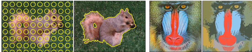
Figure 3. Binary segmentation of a color image using multivariate Gaussian distributions as region descriptor (initialization and final segmentation) and multiphase color segmentation obtained with the algorithm developed in [8].
