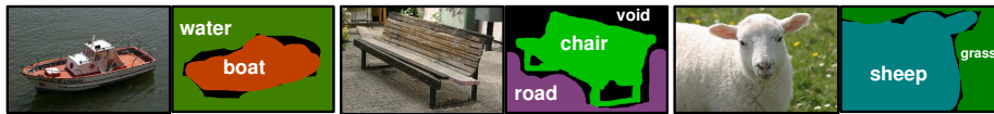
Fig. 1. The labeled image database. A selection of images in our 21-class database and their corresponding ground-truth annotations. Colors map uniquely to object class labels. All images are approximately 320 \times 240 pixels.
