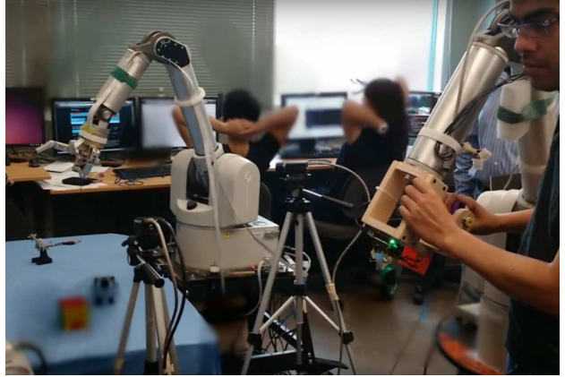
Figure 2: Tele-manipulation setup used for experimental data collection. Left: 7-DoF WAM arm with barrett hand and two eye-in-hand-cameras. Right: 4-DoF WAM arm with hand gimbal.
