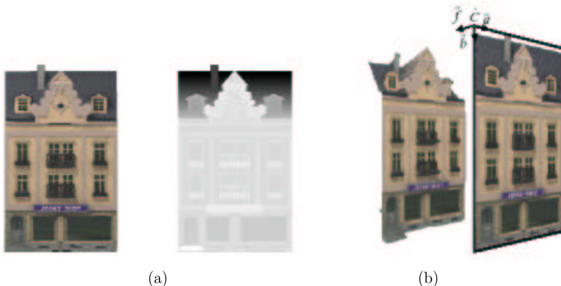
Figure 4: (a) Image texture and depth map. (b) Pre-warped relief texture and final textured and rendered house.
