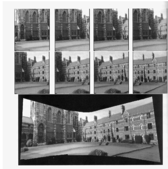
Figure 15: Eight images and the mosaic resulting from homography-based transfer
