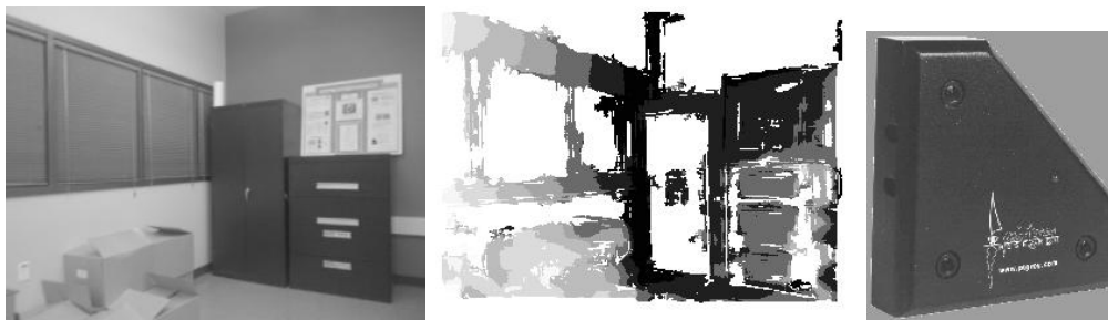
Figure 28: Example of a disparity map computed using the Triclops vision system. (a) left intensity image (b) disparity map (c) Triclops device
