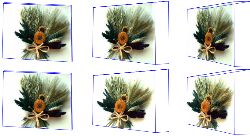
Fig. 7 Texturing a rotating quadrilateral with a wreath. Top: by warping a flat texture image. Bottom: by modulating the texture basis B and generating a continuously varying texture which is then warped onto the same quad.
