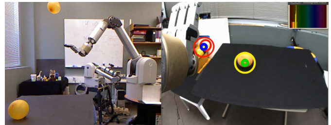
Fig. 5: Left: Eye-to-hand camera. Right: Eye-in-hand camera.
