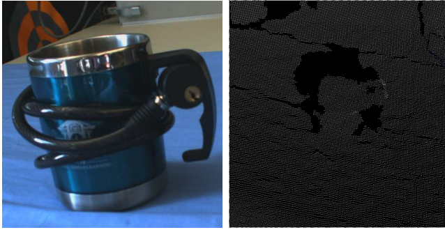
Fig. 11: Comparison of an eye in hand image of the bike lock and the corresponding point cloud.
