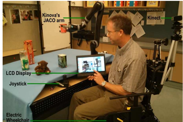
Fig. 1: Vision-based User Interface to a 6DOF robot arm and hand. By pointing and selecting in a 2D video image of the scene, the user can point to objects, select grasp types and execute robot actions. (Image edited from original to clarify that our system must be operated with both the arm and Kinect mounted on the wheelchair).
